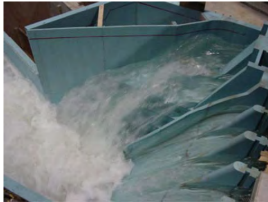
Figure 8: Flow station of hydraulic model experiment (training channel part: final design)
