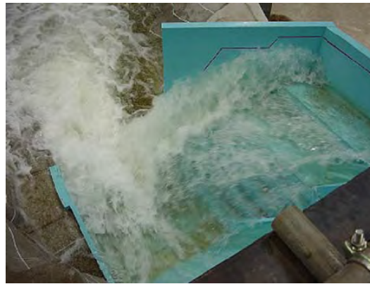
Figure 6: Flow situation of hydraulic model experiment (training channel part: original design)
